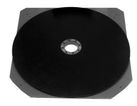
ETS-Lindgren's Model 1062-1.2B is a low profile, manually operated, nonmetallic turntable designed for pre-scan measurements. The 1062-1.2B is perfect for performing prescans, where coupling with the ground plane is not required. With a 450 kg (1,000 lb) distributed load rating, this turntable can support most EUTs that would be used with this diameter turntable. Manually rotated, the turntable can be rotated as needed, and held in position with a lock screw.
